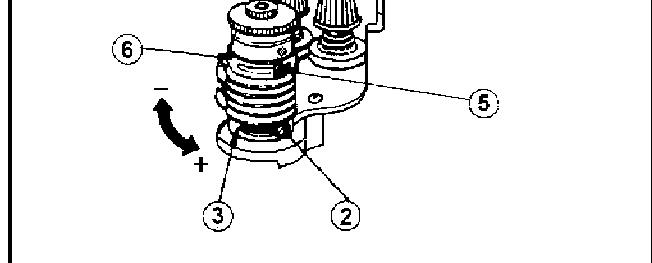
Adjusting thread position according to the sewing material. .
